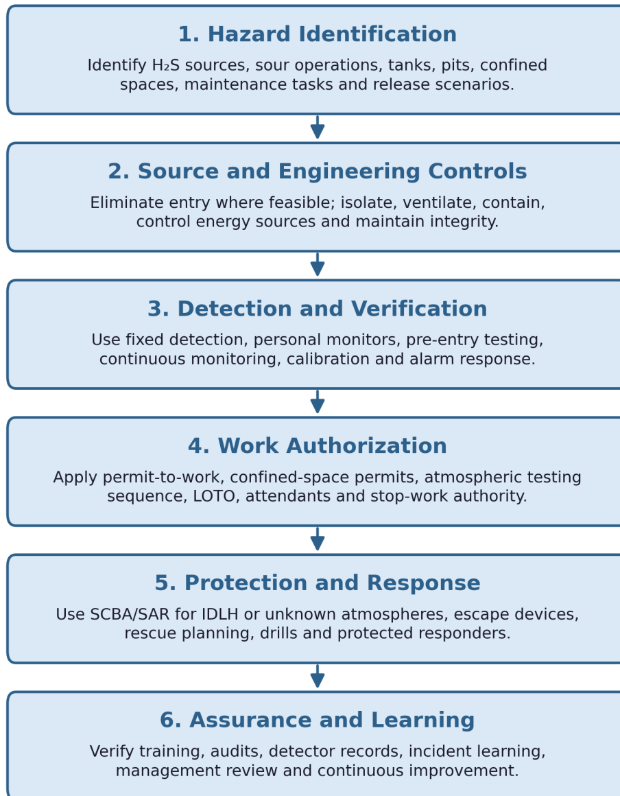
Figure 1. Barrier-based framework for H 2 S exposure risk management in oil and gas operations.
